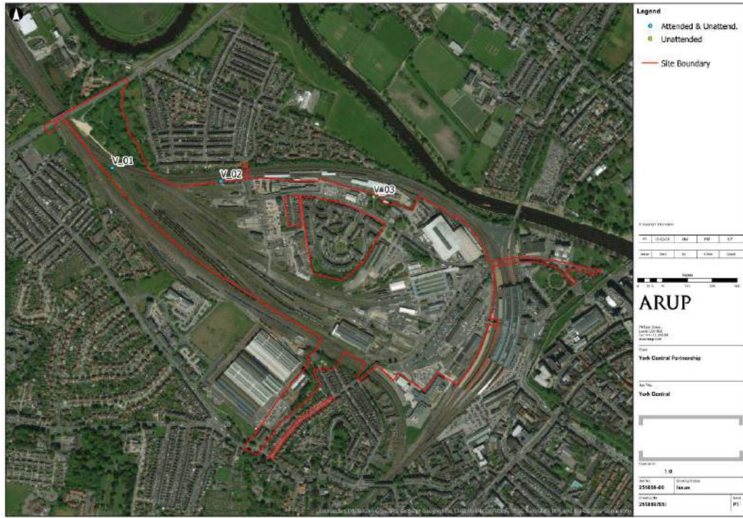
Figure 10E4: Site layout and vibration measurement locations
