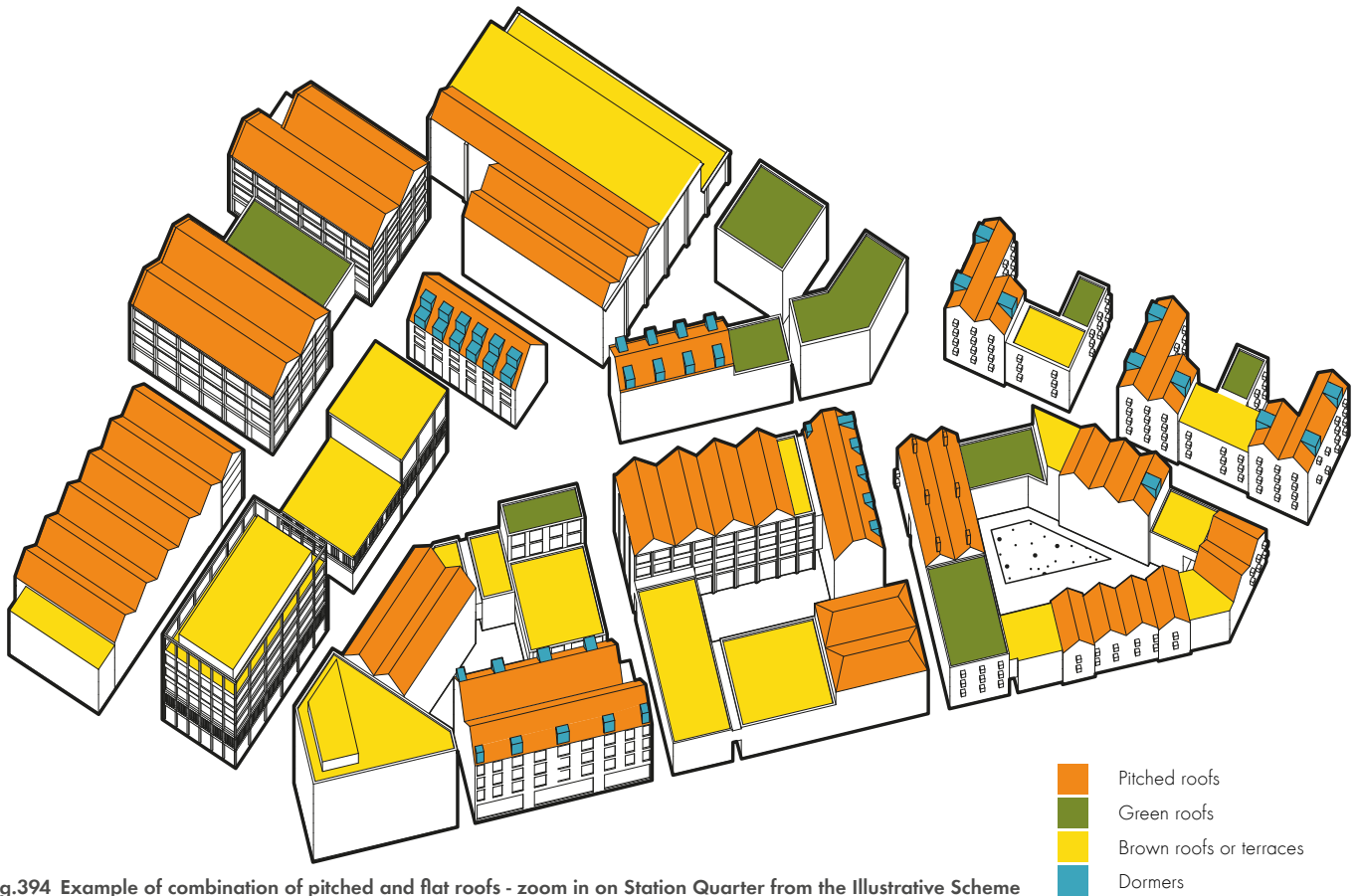
Fig.394 Example of combination of pitched and flat roofs - zoom in on Station Quarter from the Illustrative Scheme
